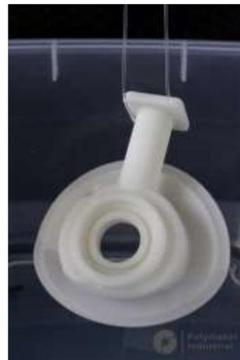
Figure 4. Dip the PolyCast™ SP802C pattern into isopropyl alcohol
